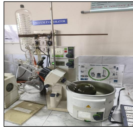
Fig.4 Rotary vacuum evaporator
