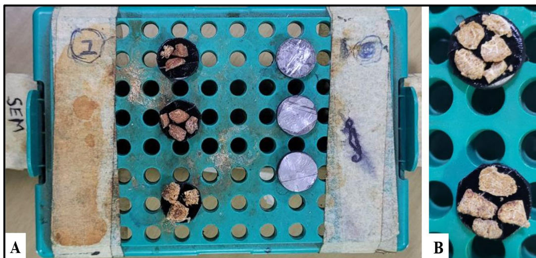
Plate 1, A & B: Photograph showing specimens mounted on aluminium stubs with double-sided carbon conductivity tape
