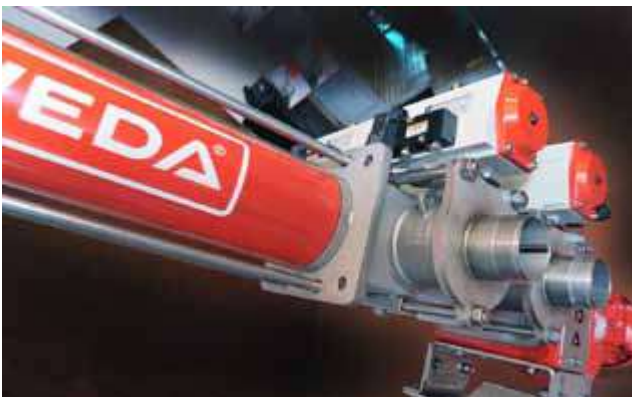
WD 15-4“: The lower the volume in the mixing zones of the extraction system, the better the hygiene situation and the lower the feed losses.
