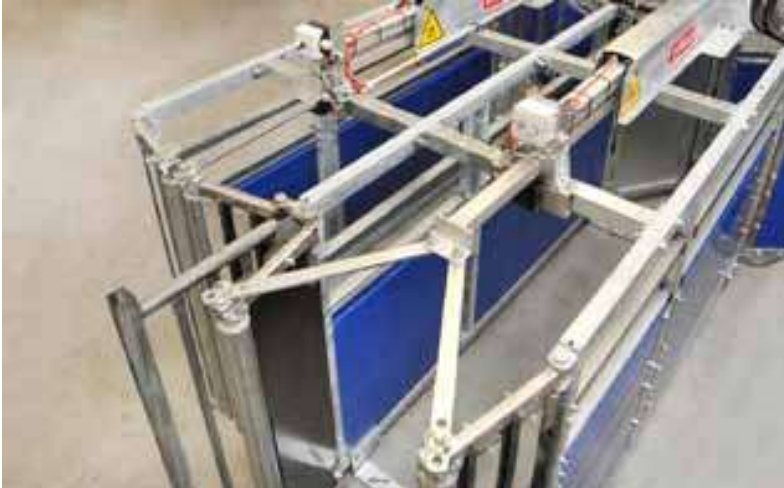
“SowComp Demand Feeding Station – Twin” of WEDA offers pig farmers the access of two groups of gestating sows to one feed trough.
